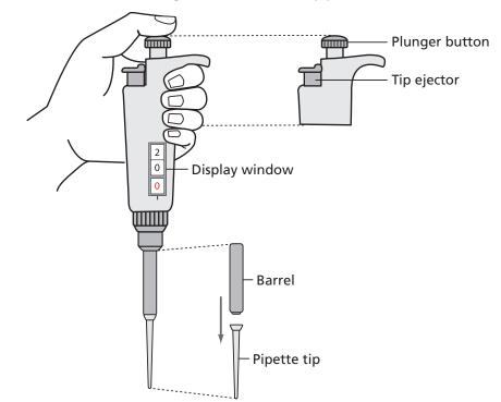
Figure 1.1: A P-20 micropipette
